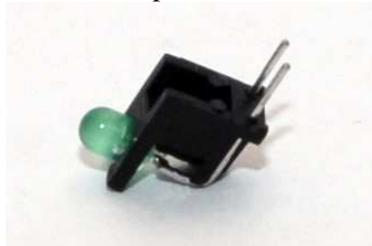
6. Install and Solder LED1 and SW1 to the board, both parts are directional and should be installed as shown below.
