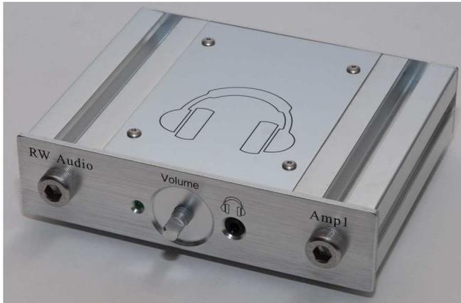
22. Now tighten all of the remaining screws holding the panels together in the order: Top – Front – Bottom – Back. Do not over tighten the 4-40 Screws, not a lot of force is required to hold them securely. Damage to the screw or allen key may result.
