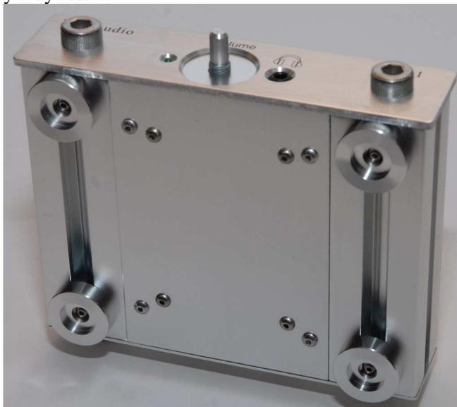
23. Move the feet to the desired locations, I suggest the front feet should rest flush up against the back of the front panel, and the back feet should sit on or just inside the back panel as shown above and below. After the screws are tightened peel off the rubber feet from the backing and install them into the recess in each foot. Turn the amp right side up and press firmly down on the amp for a few seconds to make sure the feet are properly seated.
