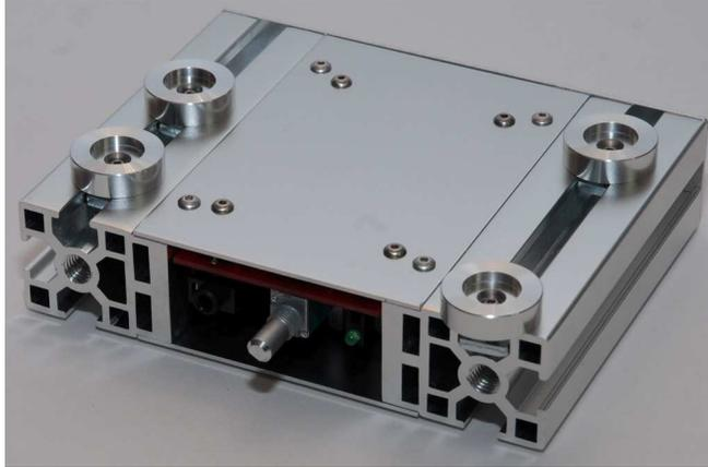
21. Install the front panel using the remaining two M8 screws. Tightening these screws should slightly recess the screw head into the pockets in the front panel as shown below. There should be no gaps around these screws and the screws should not sit on the outer face of the front panel, they should sink into the pockets.
